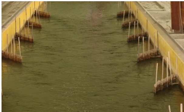
Fig 3. Bandals constructed in the laboratory rivers for navigation channel development
